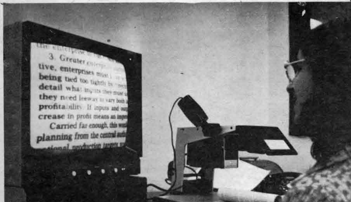
IMPROVED VISION: A visually handicapped student makes use of the Apollo Electronic visual aid to magnify reading material [Photo by Richard Schumacher].
